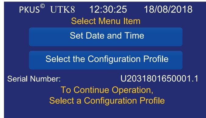
The UTK8 autonomous operation allows the configuration of test settings, carrying out all the tests provided, as well as, analyzing and archiving the test results.
