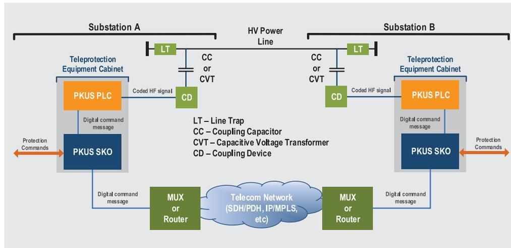
Once a failure occurs to one path, the other remains operational for protection command transmission.
