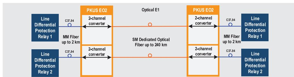
Interfacing **PKUS SKO** and Line Differential Protection Relay with C37.94 ports to one dedicated single mode optical fiber allows to use existing fiber infrastructure more effectively.
